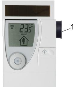
A magnet (1) is used to switch to the service level.
